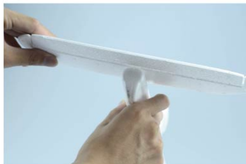
2. Bond the tailplane bonding to the body firmly
