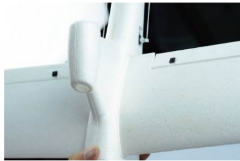
18. Ensure the wings are mounted properly NOTE: If the wings come loose after many flights, you may want to consider using a small amount of glue to hold them more securely
