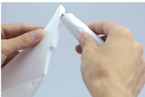
3. At the bottom of the fin evenly coat with white glue
