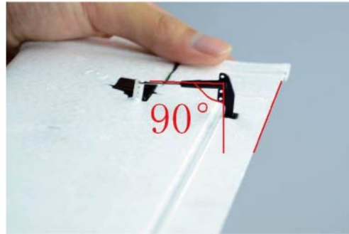
14. Adjust the servo rod and servo angle in a vertical position
