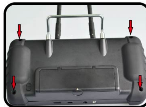
7.1. Open the cover of Transmitter by unscrewing the 4 screws as picture shows
