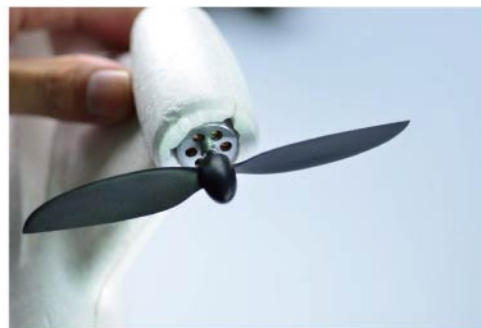
19. Screw the propellor onto the motor shaft paying attention to the thread direction. You may need to hold the motor axle with some small pliers to tighten it. Be careful not to bend or damage the motor axle if you do this.
