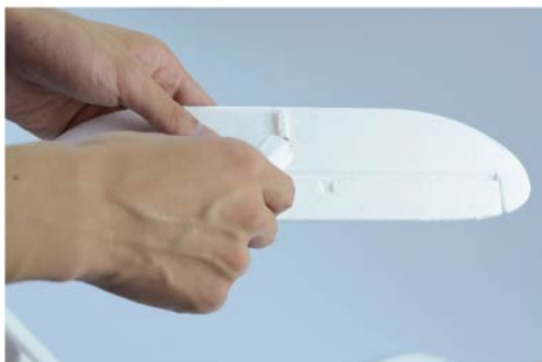
1. At the tailplane evenly coat with adhesive white glue
