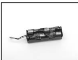
According to the correct polarities, install 8 x AA battery
