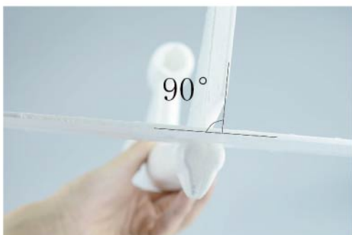
5. Adjust the fin and tailplane to a vertical 90 degree
