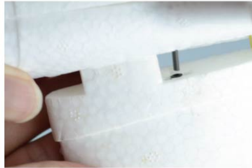
16. The two wings will meet inside the fuselage, Ensure the bolt lines up and slots together
